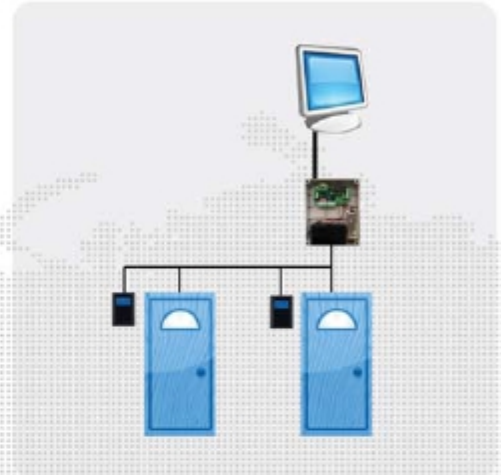
RS232 Connection Control Up To 2 Doors Configuration
